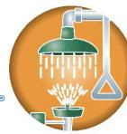
**Shower location:** The eye/facewash & body spray 8901RFK Axion must be installed in the vicinity of potential danger zones. It must be highly visible and easily accessible.
